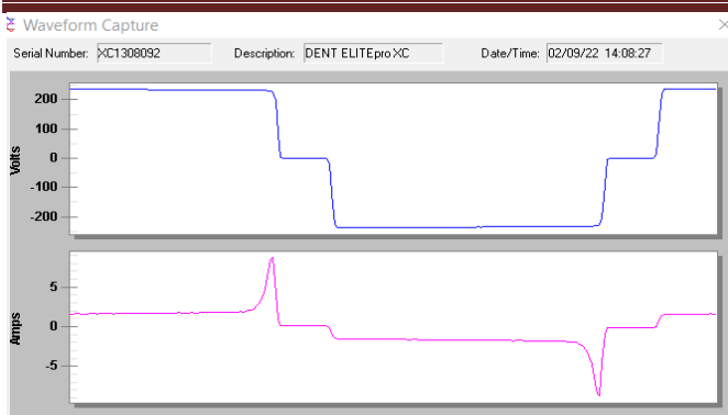
Fig. 7 (b): Voltage and Current Waveforms of the inverter output
